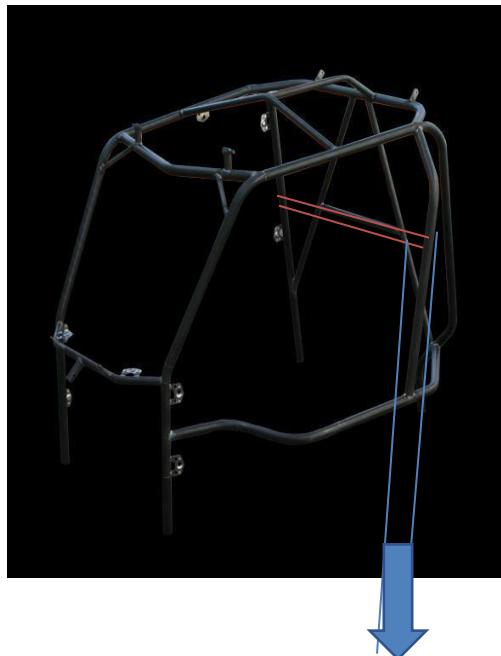
**Should a single cross tube be used it must be a minimum of 12 inches from the top of the down tube.**
